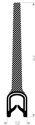
pvc + sponge rubber clamping range 1-2,5 mm roll length 50 meter
