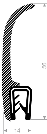
pvc + sponge rubber clamping range 1-2 mm roll length 50 meter
